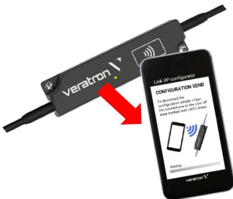
1. Launch the “Link Up Configurator” App and read the actual configuration of the LinkUp device by “tapping” the smartphone onto the LinkUp wireless area (indicated by the NFC symbol). The readout is necessary before you can write new configurations on the LinkUp.
